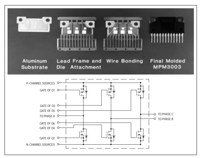
Figure 1. Construction and Diagram of the MPM3003, a Three Phase Bridge That is Ideal for Driving Small Brushless DC Motors
