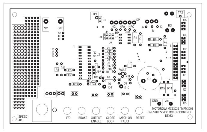
Figure 10. Printed Circuit Silk Screen of Three Phase Brushless Motor Control
