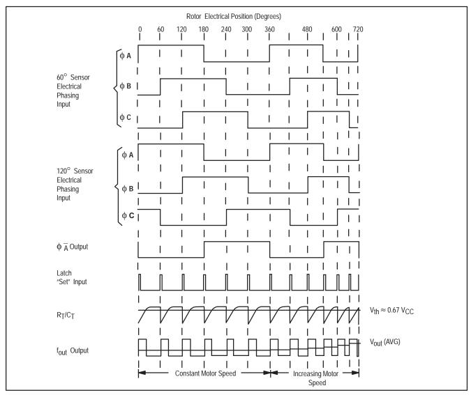
Figure 4. Timing Diagram of a Typical Three Phase, SIx Step Motor Application
