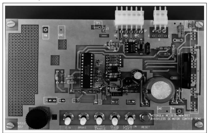
Figure 11. Brushless Motor Control Utilizing the MC33035, MC33039 and MPM3003
