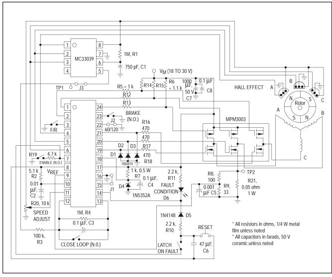
Figure 7. 24 V Brushless Motor Drive (with 120 degree sensor phasing)
