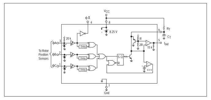
Figure 5. Representative Block Diagram of MC33039
