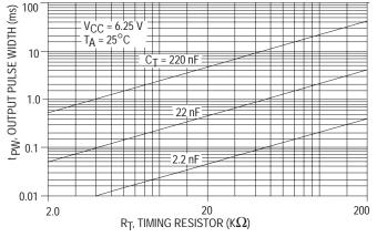
Figure 6. fout Pulse Width versus Timing Resistor
