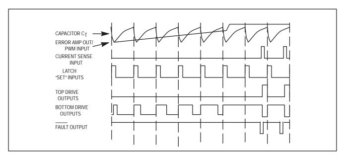
Figure 3. The MC33035's Pulse Width Modulator Timing Diagram
