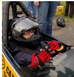
Driver ready to race before an event. Notice the harness, helmet, gloves and roll cage for driver safety.
