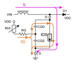
• V<sub>TH</sub> is exceeded and MOSFET starts conducting in linear mode:
