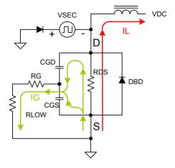
Turn-off time can be estimated using Q<sub>Q,SR</sub> as determined in [3]
