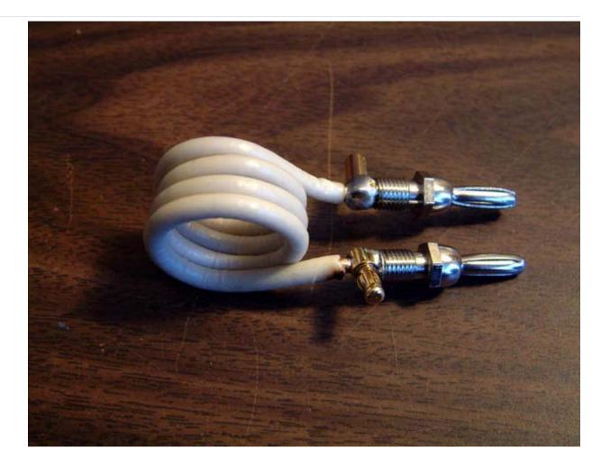
Now you are done! Pretty easy huh! If you want, you can add some short lengths of wire just above the banana plugs and crimp or solder your battery connectors to these leads. The important measurement is that the current must travel through 12 inches of 10ga wire to be accurate, so be sure to atttach your wires right up next to the insulation on the 10ga wire.
