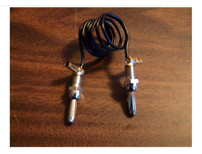
To use the shunt, plug it into the voltage and ground holes on your DVM as shown below. Make sure that the connector that mates into the battery goes into the voltage hole, and the connector that mates with the speed controller goes in the ground hole. (If you get it backwards it will still work, it will just display a negative value) Turn the voltmeter to the lowest voltage scale, usually 200mV or 300mV. The one in the photo below has a 200mV scale.
