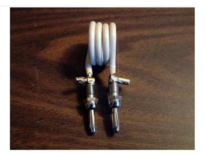
I repeated the process using a piece of solid 18ga wire that was 18.79 inches long. This form a current shunt that reads 10 millivolts per amp. Here is a photo of this one.
