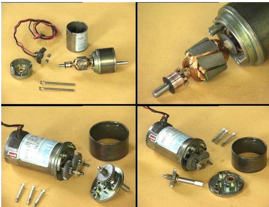
Pittman GM8712 disassembly of motor and gearhead
