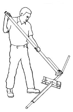
Operation of the pending tool is relatively easy. The pipe that you wish to create a bend in is placed in the clamp and the two nuts are tightened to ensure that the pipe does not slip. One the pipe is clamped up the bending arm can be slipped onto the pipe and positioned appropriately. The long arm of the tool makes the job of bending the pipe easy.
