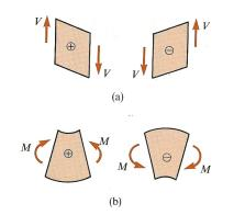
Positive shear forces always deform right hand face downward with respect to the left hand face. Positive bending moments always elongate the lower section of the beam.
