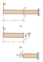
It is convenient to reduce the resultant to a shear force, V, and a bending moment, M. Because shear forces and bending moments are the resultants of stresses distributed over the cross section, they are known as **stress resultants** and in statically determinate beams can be calculated from the equations of static equilibrium.
