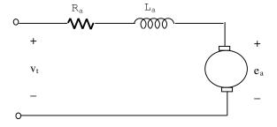
Ra - lumped armature winding resistance
