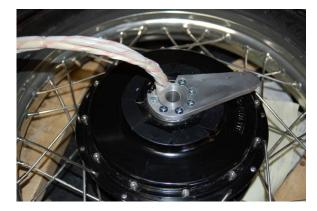
This is a picture of the torque are on the wire side.
