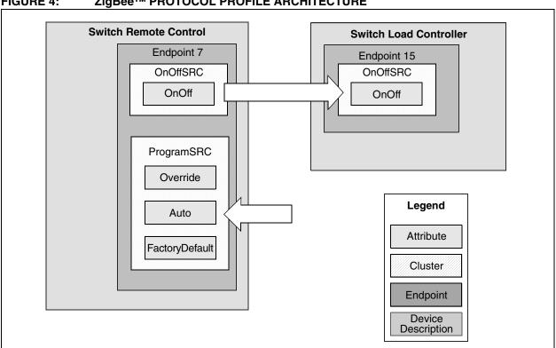
FIGURE 4: ZigBee™ PROTOCOL PROFILE ARCHITECTURE
