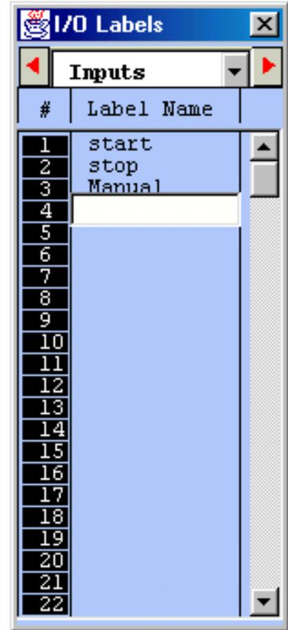
4. Enter the name "Start" for Input #1. Press <Enter> key to accept the name. The text field will be closed and the name "Start" is now assigned to Input #1. If you made a mistake, simply press the "spacebar" or click on the input location again to edit it.
