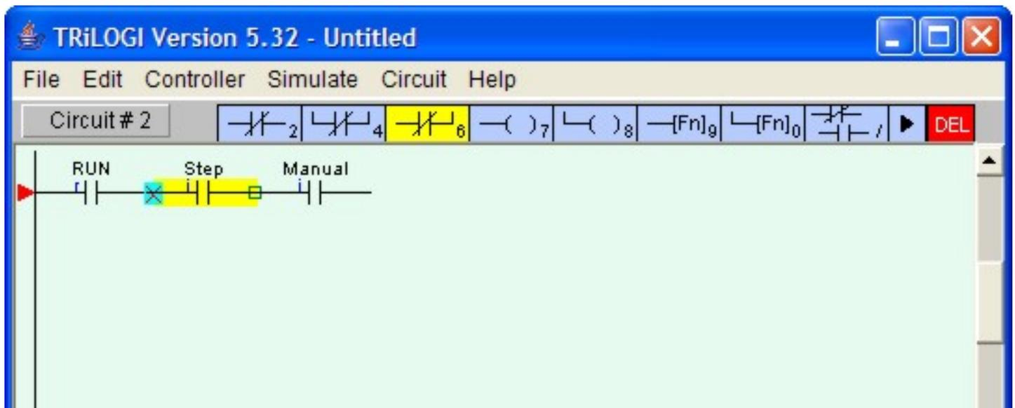
2. We want to enclose the two series contacts "Step" and "Manual" with a parallel branch that contains two elements. First, we will create the branch for the N.C. "Manual" contact.
