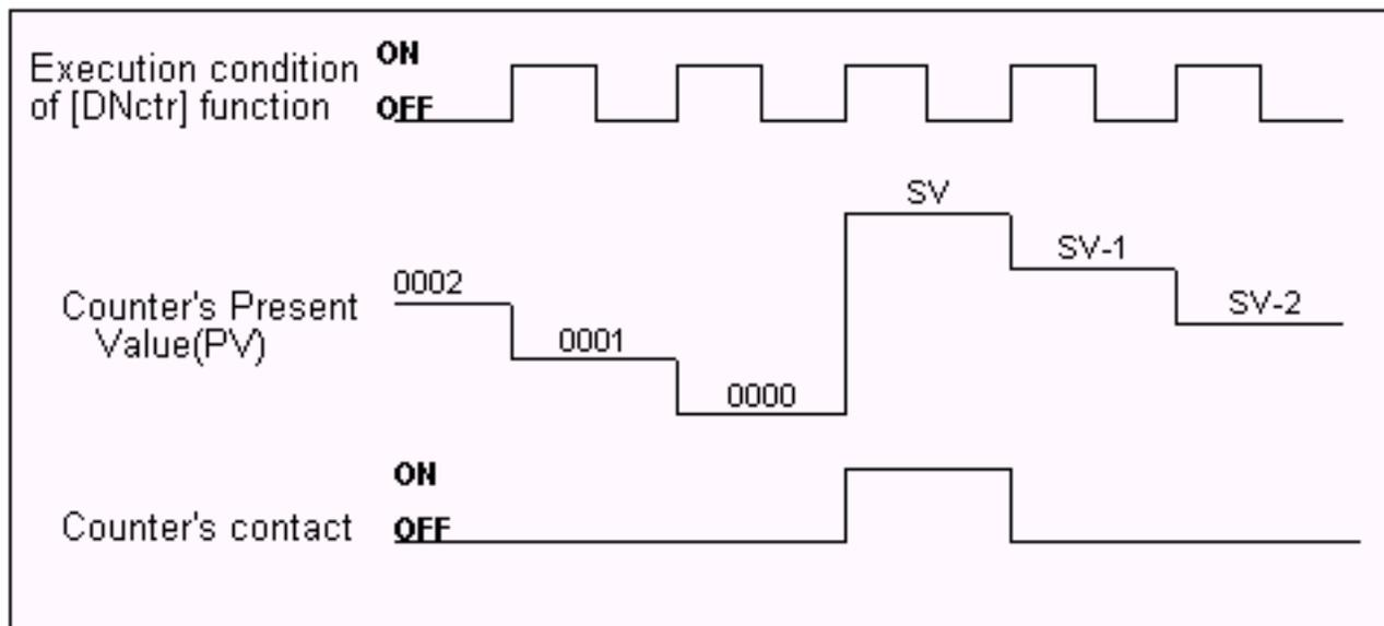
Each time when the execution condition of a [DNctr] function changes from OFF to ON, the present value of the designated counter is changed as follow:
