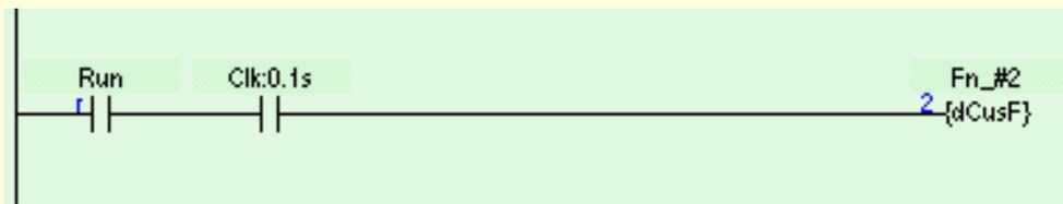
For example, you don't need to update the value of a variable displayed on the LCD screen any faster than the human eye can read them. So using a 0.5s clock pulse may be sufficient and this will not take up too much CPU time for the display. For slow processes such as heating, a 1.0s clock pulse to monitor temperature change is more than sufficient.
