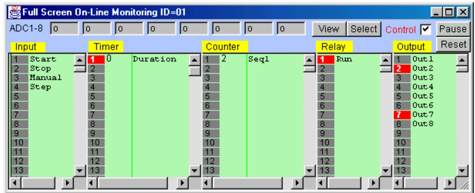
The Full Screen Monitoring screen comprises 5 columns: Input, Timer, Counter/Sequencer, Relay, and Output. With the exception of the Relay table which contains up to 512 elements, all other columns contain 256 elements each and each one has a vertical scroll bar. You can use the mouse to scroll each column independently to locate the desired I/O.
