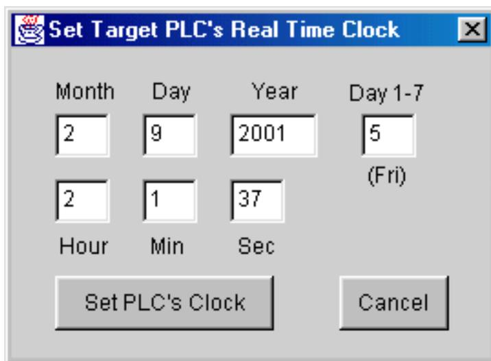
The dialog box will be closed after the TRiLOGI has transferred all the data to the PLC. You should use on-line monitoring to verify that the data has indeed been properly written into the PLC.
