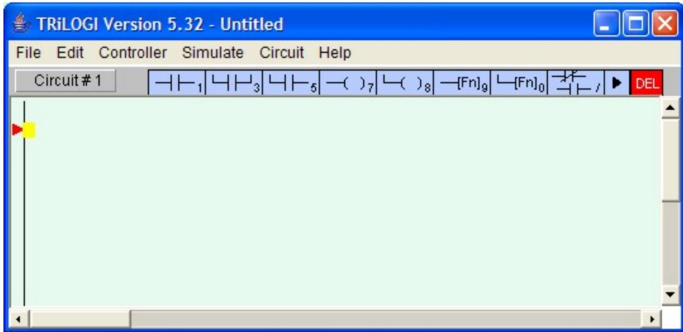
Once you enter the "Ladder Edit" mode, a row of ladder icons appear along the top of the main TRiLOGI window just below the pull down menu. The following is a description of each item. A yellow color highlight bar, which you can move to select an element in the ladder circuit, will appear.
