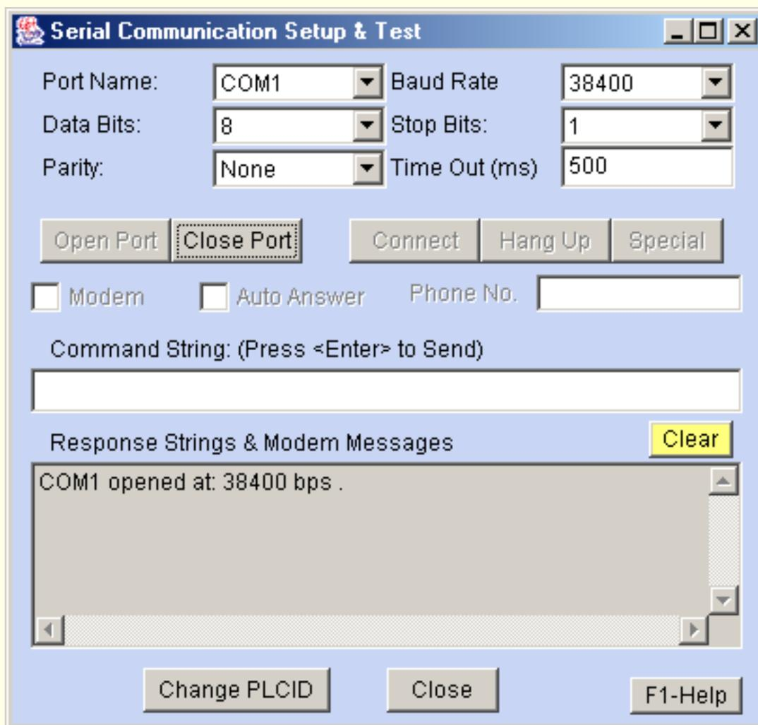
This dialog box allows you to configure the serial port of the host computer to match the setting on the PLC for proper communication. Most of the items here are self-explanatory. If you have more than one PLC connected to the host computer via RS485, all the PLCs must have the same serial port settings as the TLServer. The **Open Port** button allows you to test whether the
