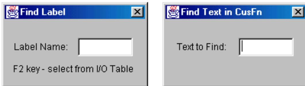
**Find Ladder element:** you can enter into the the text field a string that partially or fully matches the label name you wish to locate. You can also press the <F2> key to open up the I/O table and pick the label name from the I/O table.
