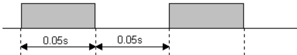
The clock pulse bits are often used with counter instructions to create timers. Additionally, they can be used as timing source for "Flasher" circuit. A reversible counter can also work with a clock pulse bit to create secondary clock pulses of periods that are multiples of the basic clock pulse rate.
