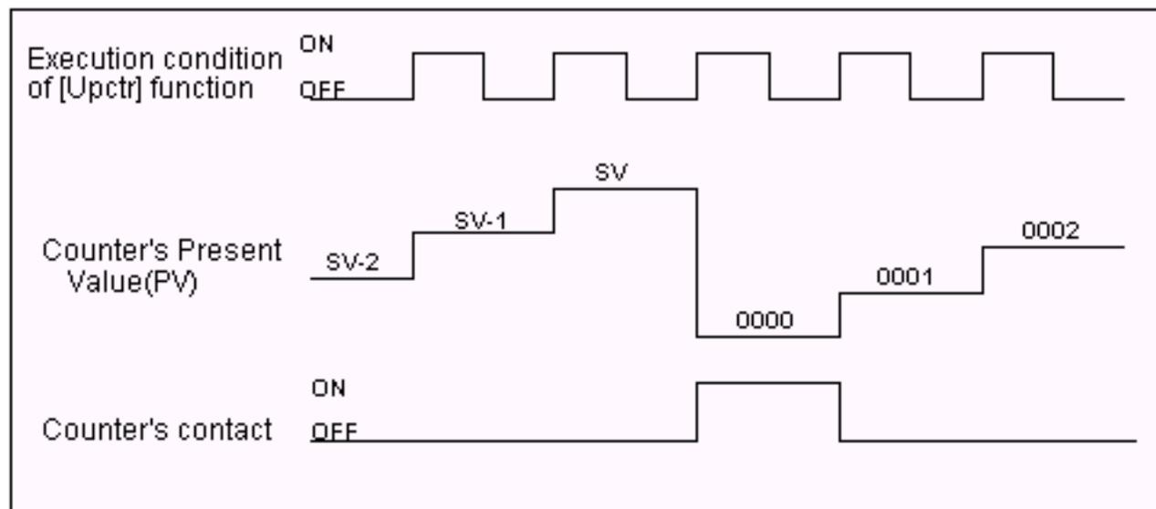
Each time when the execution condition of an [Upctr] function changes from OFF to ON, the present value of the designated counter is affected as follow:
