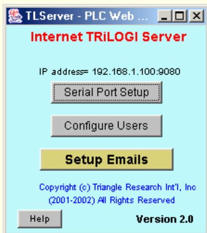
**TLServer** acts as a gateway to connect the M-series PLC to the corporate LAN or the Internet so that they can be controlled and programmed by a TRiLOGI client from anywhere in the world.
