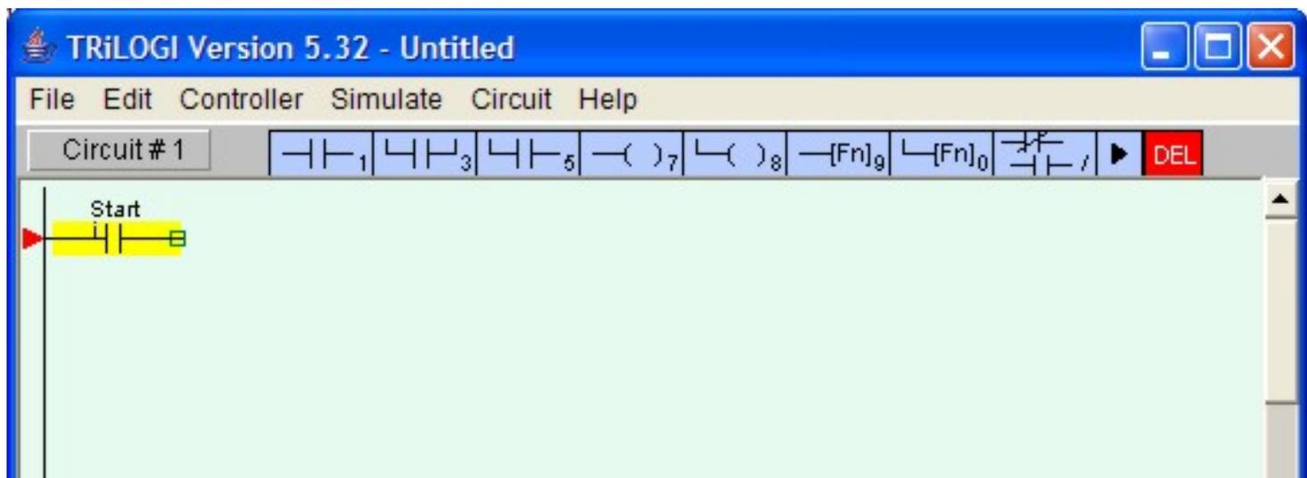
If you observe the highlight bar carefully, you will notice a dark green color square at the right end of the highlight. This indicates the insertion location where a series contact will be attached. You can change the insertion location to the left or the right of the highlight bar by pressing the **<SHIFT>** key or **<TAB>** key (Note: **<TAB>** key only works on JRE 1.3.1 or earlier. It does not work on JRE 1.4.x)
