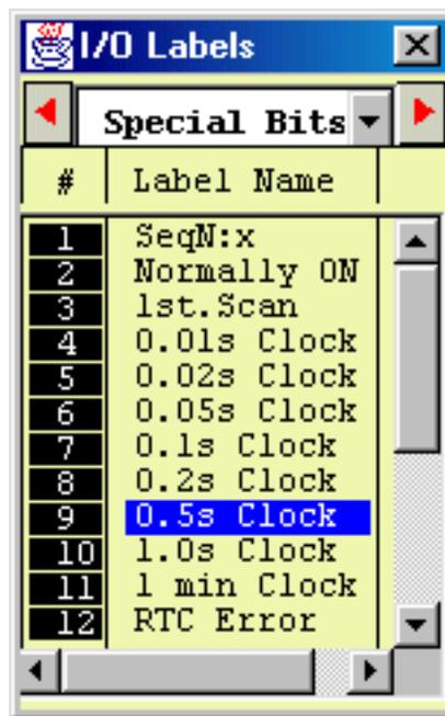
The "Special Bits" table is located after the "Counters" table and before the "Inputs" table. Then click on the "SeqN:x" item to insert a sequencer bit. You will be prompted to select a sequencer from a pop-up menu. Choose the desired sequencer (1 to 8) and another dialog box will open up for you to enter the specific step number for this sequencer.
