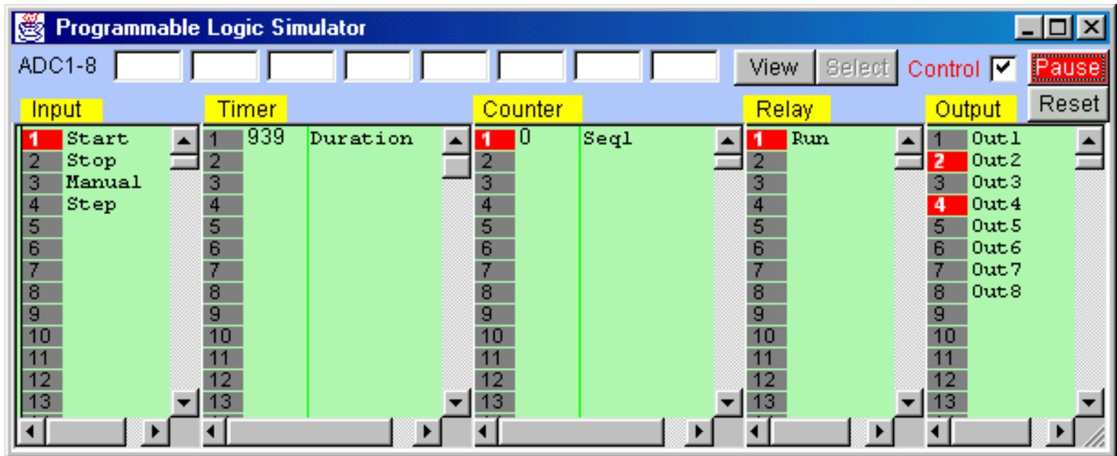
The simulator screen comprises 5 columns: Input, Timer, Counter/Sequencer, Relay, and Output. With the exception of the Relay table which contains up to 512 elements and the timer table which contain up to 128 elements, all other columns contain 256 elements each and has a vertical scroll bar. You can use the mouse to scroll each column independently to locate the desired I/O.
