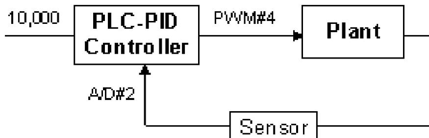
E.g. Implementing Closed-Loop Digital Control with PID computation function
