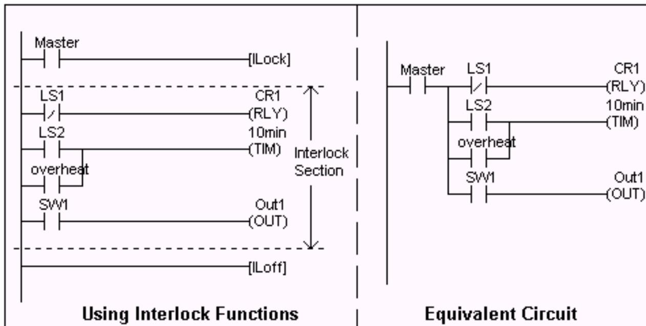
Note that [LOff] is the only function that does not need to be energized by other program elements. When you use one or more [ILock] functions, there must be at least one [LOff] function before the end of the program. Otherwise the compiler will warn you for the missing [LOff]. The logic simulator always clears the Interlock at the end of the scan if you omit the [LOff] function.
