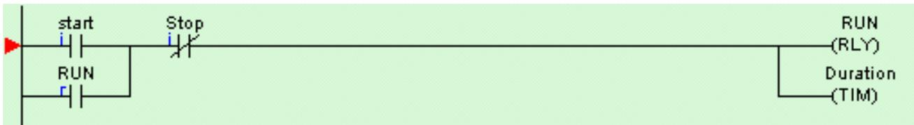
1. With the circuit pointer (red color triangle) at Circuit #1, press the <Spacebar> to enter the "Ladder Edit" mode. You can also enter the circuit edit mode by double clicking at Circuit #1.
