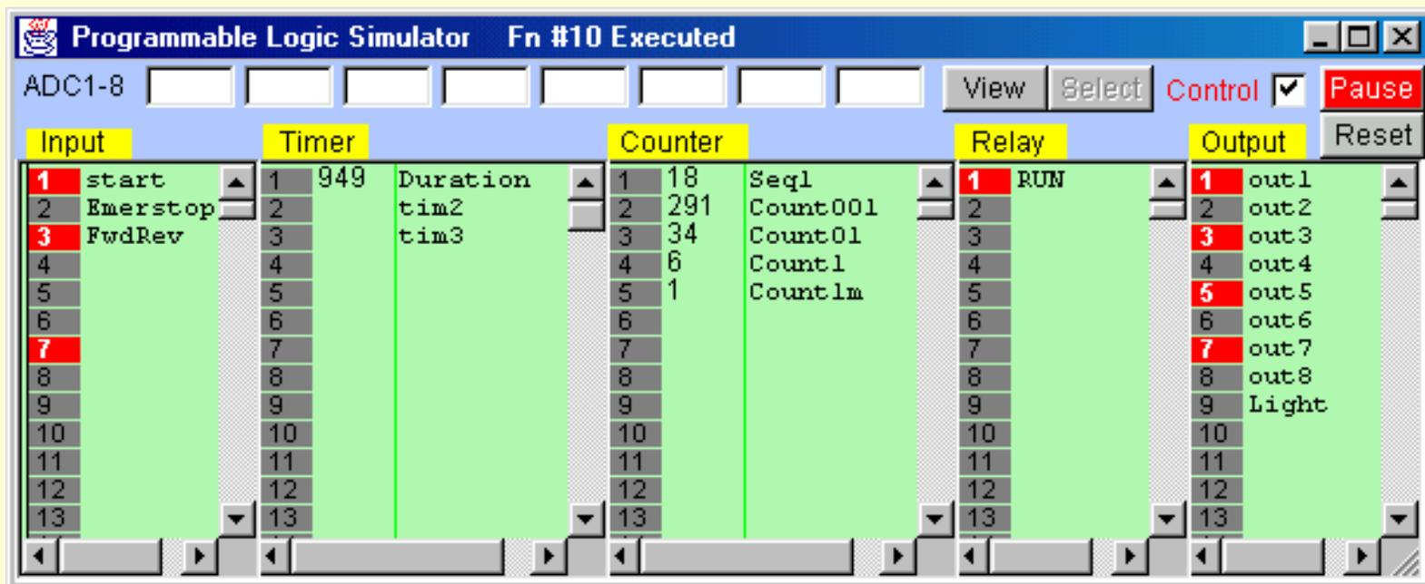
An I/O or internal relay bit that has been turned ON is indicated by a RED color rectangular lamp that simulate a LED being turned ON. You can pause the logic simulator at any time by pressing the <Ctrl-P> key or clicking on the [Pause] button. Likewise the simulator engine can be reset by clicking on the [Reset] button.
