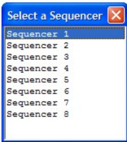
8. When prompted, select Sequencer 1. This function will increment the step counter of Sequencer #1 each time its execution condition goes from OFF to ON.
