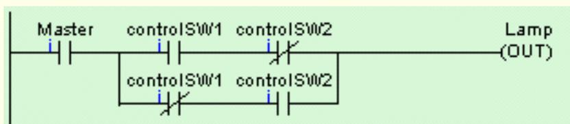
A contact with a "/" across its body is a **Normally-Closed (N.C.) contact**. What it means is that the ladder program is using the "inverse" of the logic state of the input to interpret the diagram.
