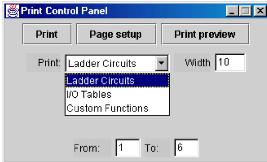
To print, first select the item from the choice box and define the range you wish to print and then click on the "Print" button. For "Ladder Circuits", the range indicates the circuit numbers. For "I/O Tables", the range indicates the I/O number (up to 256) and for "Custom Functions", the range is the function number.
