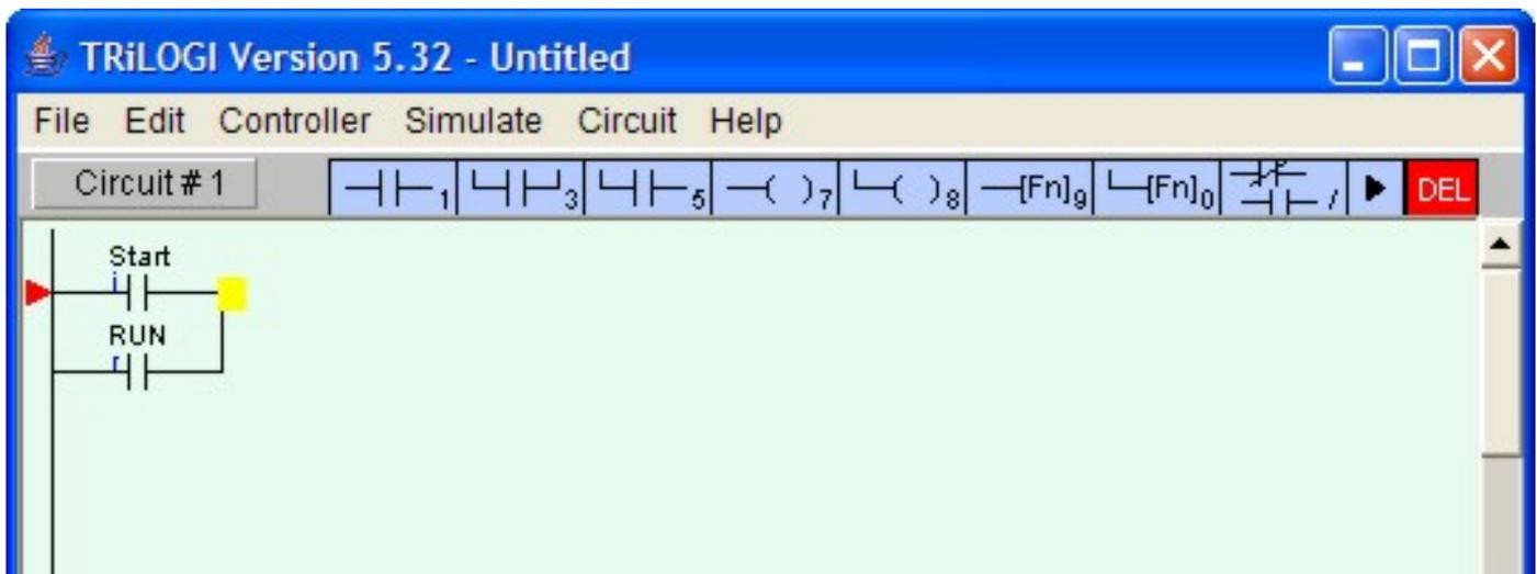
Note: In TRiLOGI Version 5.32 or higher, the highlight bar will move to the junction if you click on the dark green insertion point on the "Start" contact.
