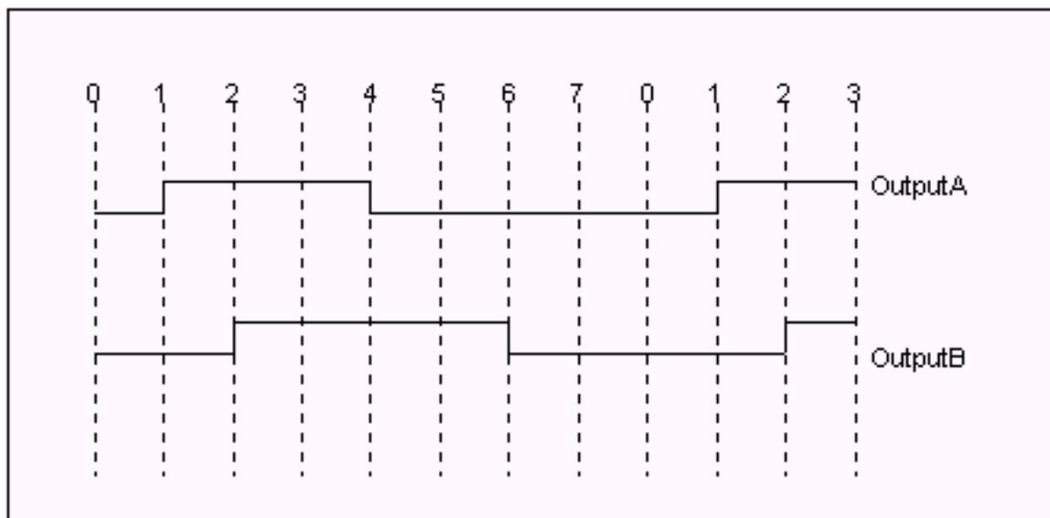
This can be replaced by an 8-step sequencer. Step 1 (e.g "Seq1:1") turns ON and latch Output A using [Latch] function, Step 2 turns ON and latch Output B, Step 4
