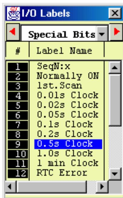
The "Special Bits" table is located after the "Counters" table and before the "Inputs" table. Then click on the "SeqN:x" item to insert a sequencer bit. You will be prompted to select a sequencer from a pop-up menu. Choose the desired sequencer (1 to 8) and another dialog box will open up for you to enter the specific step number for this sequencer.
