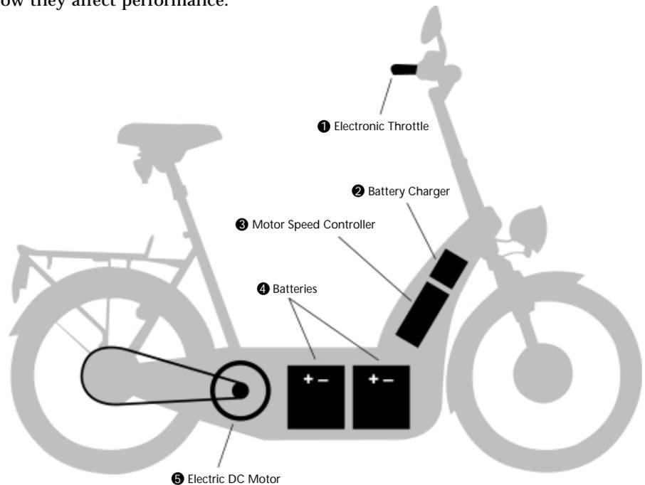
**1-ELECTRONIC THROTTLE** The throttle for a quality electric vehicle sends an electronic signal to the motor controller allowing the rider to precisely and smoothly change and control speed. On budget PEVs, an on/off switch is used.
