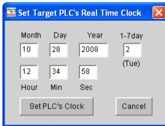
Figure 12.1: Set Real Time ClockSetting the RTC Using TBASIC
