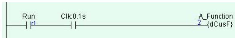
For example, you don't need to update the value of a variable displayed on the LCD screen any faster than the human eye can read them. So using a 0.5s clock pulse may be sufficient and this will not take up too much CPU time for the display. For slow processes such as heating, a 1.0s clock pulse to monitor temperature change is more than sufficient.
