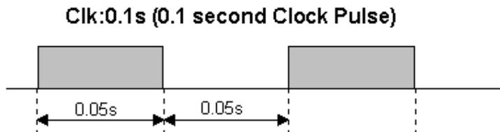
The clock pulse bits are often used with counter instructions to create timers. Additionally, they can be used as timing source for "Flasher" circuit. A reversible counter can also work with a clock pulse bit to
