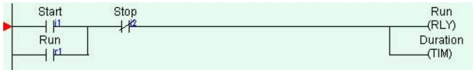
18. With the circuit pointer (red color triangle) at Circuit #1, press the <Spacebar> to enter the "Ladder Edit" mode. You can also enter the circuit edit mode by double clicking at Circuit #1.
