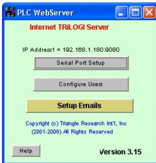
**TLServer** acts as a gateway to connect the M-series (or F-series) PLC to the corporate LAN or the Internet so that they can be controlled and programmed by a TRiLOGI client from anywhere in the world.
