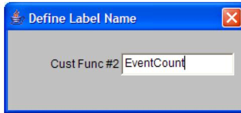
Note: For custom function only, it is possible to create a custom function without defining its label name. If you leave the text field empty the program will give the custom function a default name: Fn\_#n where n is the function number which varies between 1 and 256.
