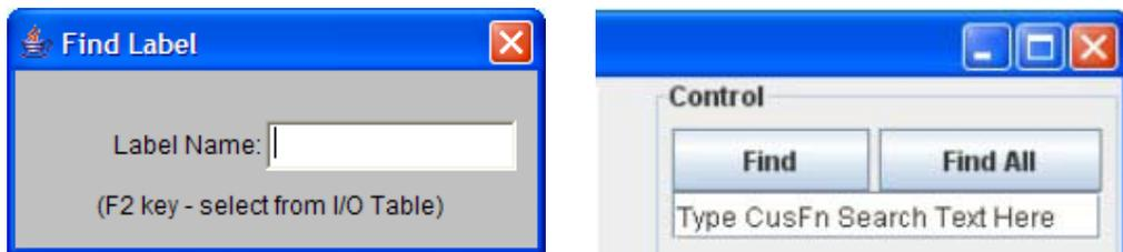
**Find Ladder element:** you can enter into the text field a string that partially or fully matches the label name you wish to locate. You can also press the <F2> key to open up the I/O table and pick the label name from the I/O table.
