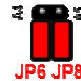
A4 and A5 are configured to be used as I2C communication lines (A4 – SDA, A5 – SCL )
