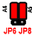
A4 and A5 on J7 are configured to be used as analog inputs
